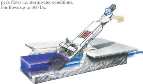
The SPIROGUARD Double Channel Screen design eliminates problems with sedimentation at the channel bottom during periods of low flows.
